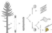
Material Inventory Inventory of unique short timber lengths is generated from naturally occurring tree branch geometry
